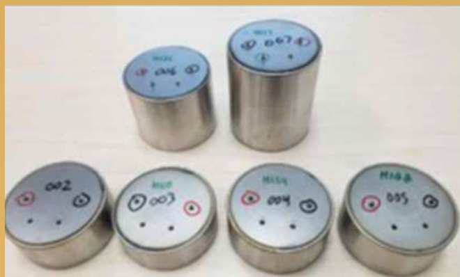
Test battery hardware: High temperature thermal batteries adapted for the Venus surface. Image Credit: Dr. Michael Barclay, Advanced Thermal Batteries, Inc.
