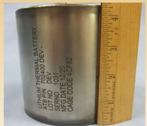
1/3 scale developmental battery developed by Advanced Thermal Batteries, Inc. for LLISSE. Image Credit: Tom Miller, NASA GRC
