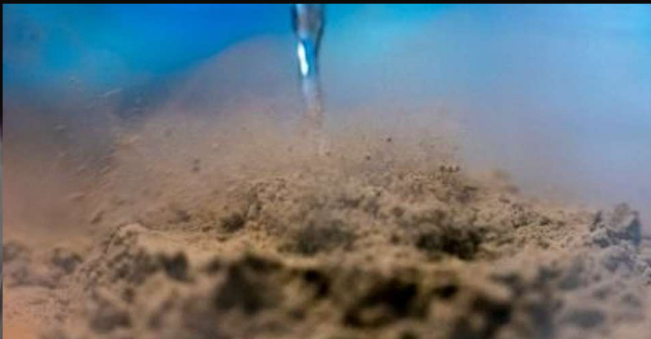
A close-up image of a dropper releasing liquid nitrogen on a pile of volcanic ash. (Image credit: Ian Wells)
