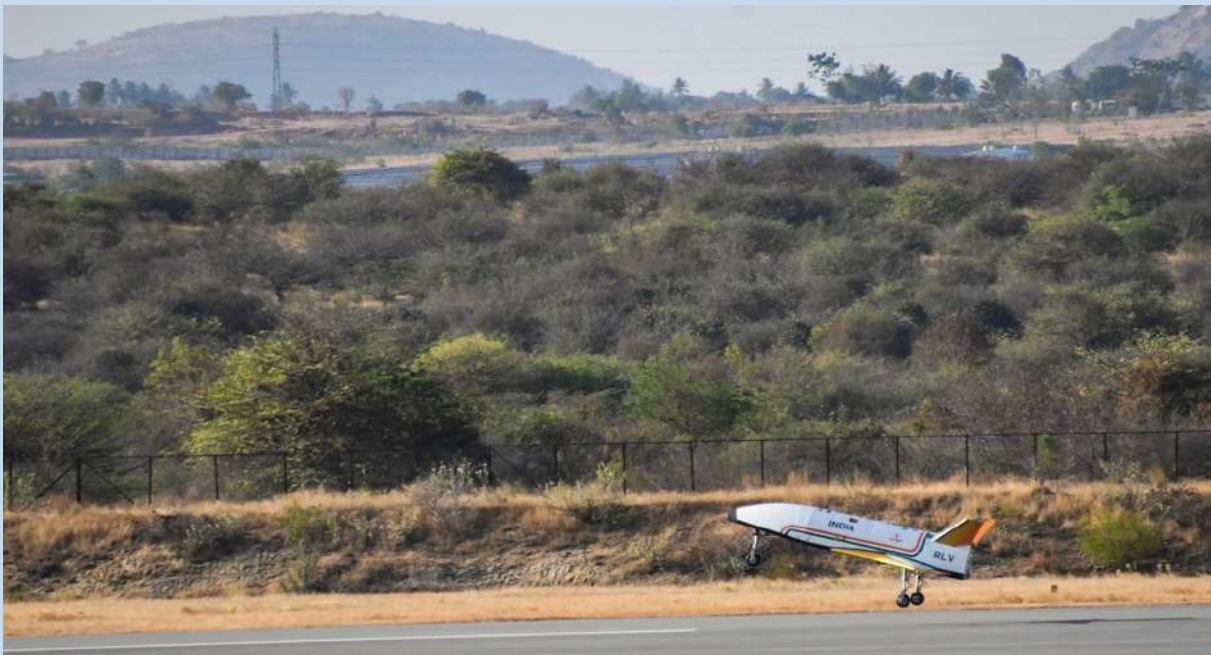
India's reusable space plane prototype comes in for a landing on April 2, 2023 after a drop test.
