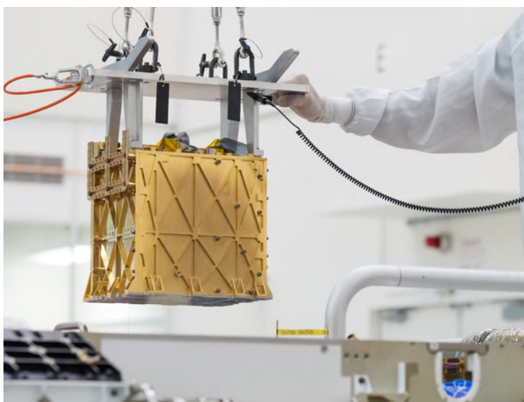
The Mars Oxygen In-Situ Resource Utilization Experiment (MOXIE) instrument is lowered into the Perseverance rover, March 21, 2019 at NASA's Jet Propulsion Laboratory, in Pasadena, Calif.
