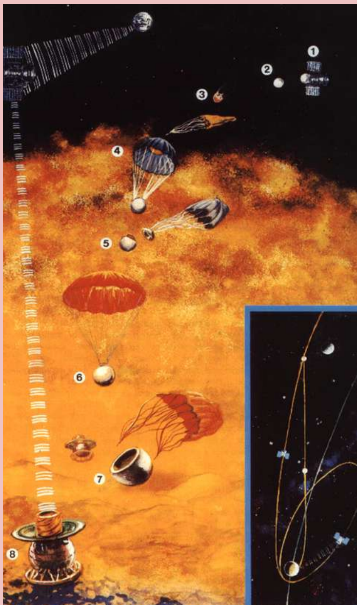
A 1962 diagram of the Venera probe and the landing sequence for the Soviet Union's Venera spacecraft (Credits: NASA)
