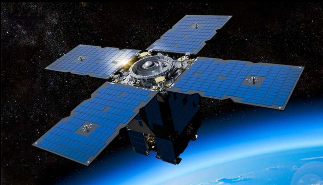
The most precise clock ever flown in space, NASA's Deep Space Atomic Clock, could improve spacecraft navigation throughout the solar system. This illustration shows the spacecraft carrying the clock.
