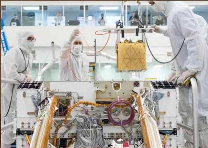
MOXIE (Mars Oxygen In-situ Resource Utilization Experiment) is lowered into the chassis of NASA's Perseverance in 2019. During the mission, MOXIE extracted oxygen from the Martian atmosphere 16 times, testing a way that future astronauts could make rocket propellant that would launch them back to Earth.
