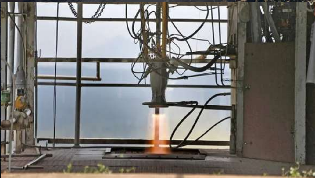
A PS4 engine, used in the upper stage of India's PSLV rocket, undergoes hot-fire testing on May 9, 2024. The engine was built using additive manufacturing, in a potential breakthrough for Indian rocket technology. (Image credit: ISRO)
