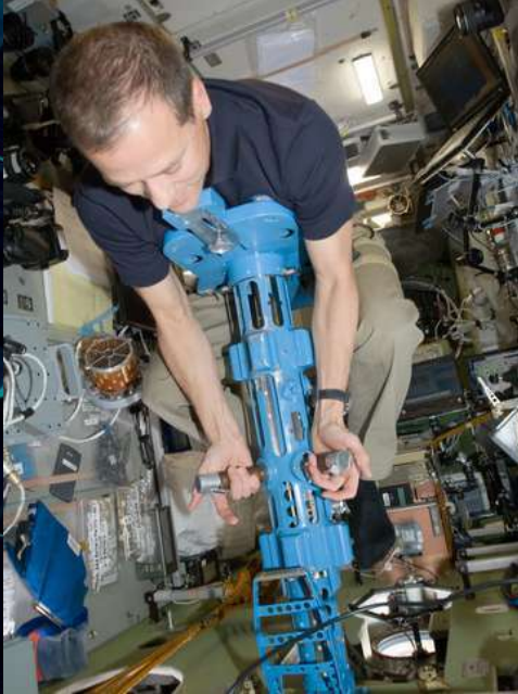
NASA astronaut Tom Marshburn uses the Body Mass Measurement Device in the Zvezda service module aboard the International Space Station on Dec. 23, 2012. (Image credit: NASA)
