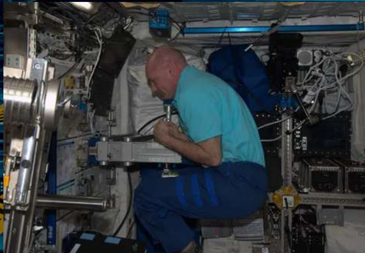
European Space Agency astronaut André Kuipers uses SLAMMD to measure his body mass. (Image credit: NASA/ESA)
