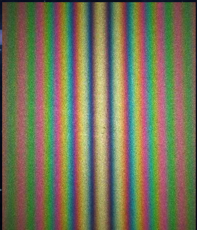
Fringe Pattern produced with a Michelson interferometer using white light. (Credit: Alain Le Rille)
